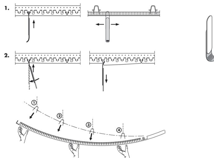
**GB** Demounting the panels shall only be done utilising the special demounting tool. Any other tool may damage the panels. While demounting the panel make sure to support the part of the panel that has already been removed from the carriers.
